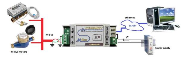
Typical wiring of the converter with M-Bus devices, power supply and Ethernet network connection.
